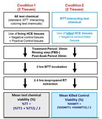
Case by case test conditions for HPLC/UPLC-spectrophotometry endpoint
